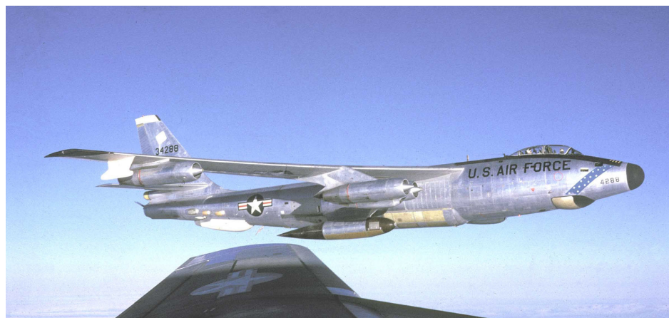
An RB-47 in flight. Note the various bumps/blisters on the underside of the aircraft and wings. (Source: USAF)
